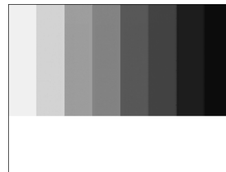
Figure 4-71. Split Field Color Bar, 625 Line Systems
