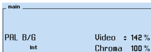
Figure 4-24. Video Amplitude Stepping
